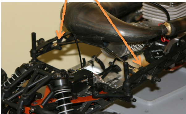
Exhaust supported by body mount pins
